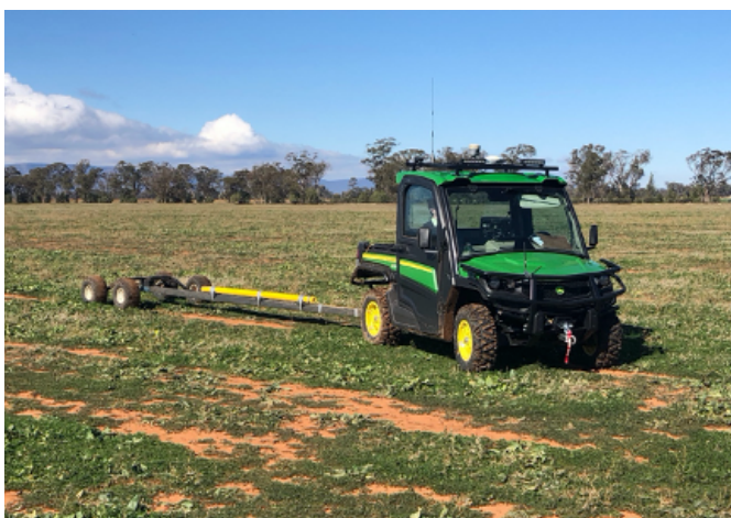
Electromagnetic survey (soils assessment) at Tomingley 8 July 2020
