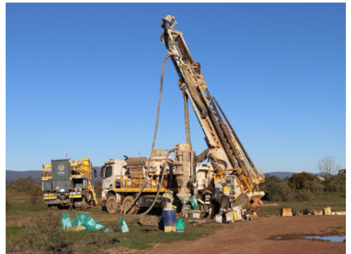
Strike Drilling working on the resource assessment at Roswell.
