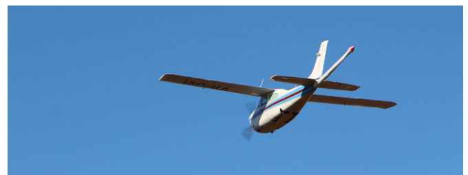
The survey involved a small aeroplane flying approximately 35-40 metres above the land surface.
