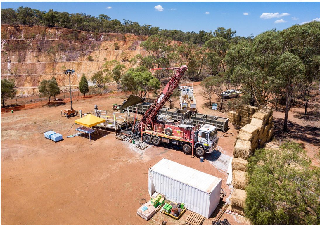
Drilling at Peak Hill Gold Mine in January. Mitchell Services diamond drill rig behind a sound bund of wheaten hay. (Photo courtesy Mitchell Services)
