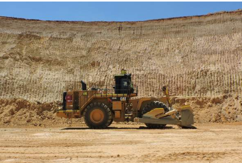
New 854 wheel dozer onsite in the Caloma pit helps manage noise
